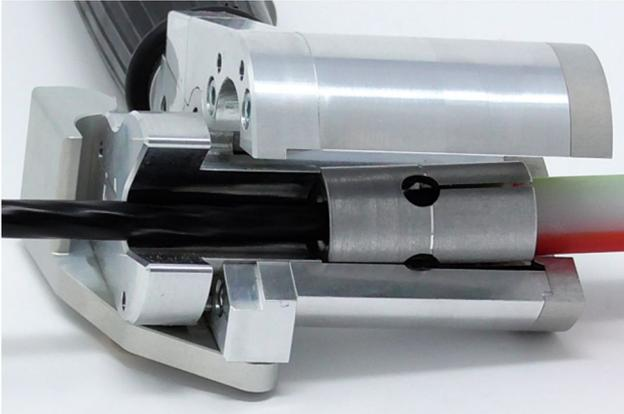
5.1 Put WGT into assembly pliers and close it. Cable has to point out top side of tool, micro duct has to point out to bottom side. If it doesn't close perfect, WGT was inserted faulty.
