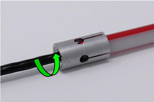
3.6 Release WGT by turning counterclockwise but hold cable during procedure.
