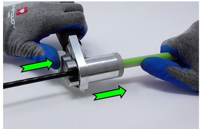
4.4 Press release lever and push WGT onto micro duct.
