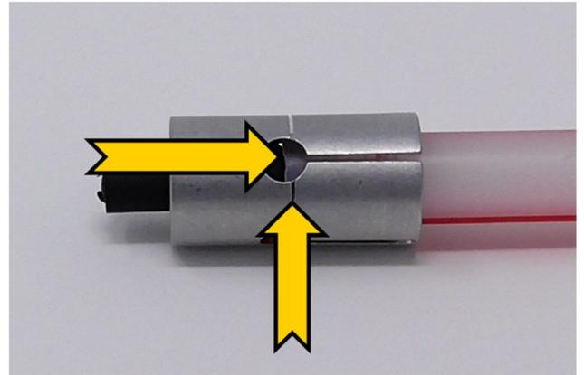
1.5 Push WGT on the micro duct until the edge of the duct is at least flush with the ring marking on WGT body (arrows). This ensures tightness of WGT.
