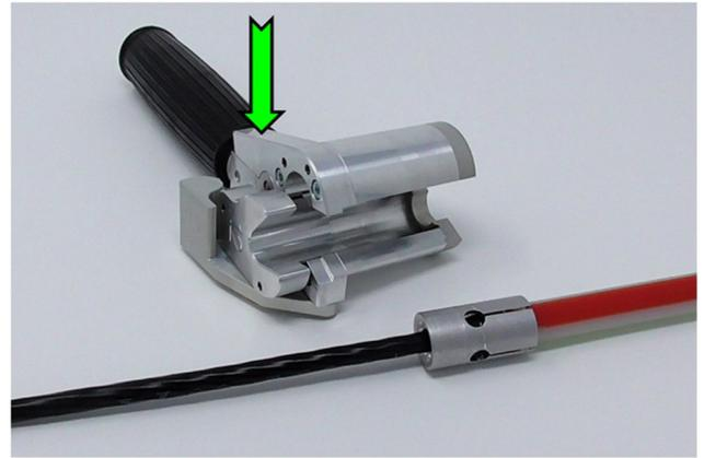
4.2 Open assembly pliers by pushing opening lever.
