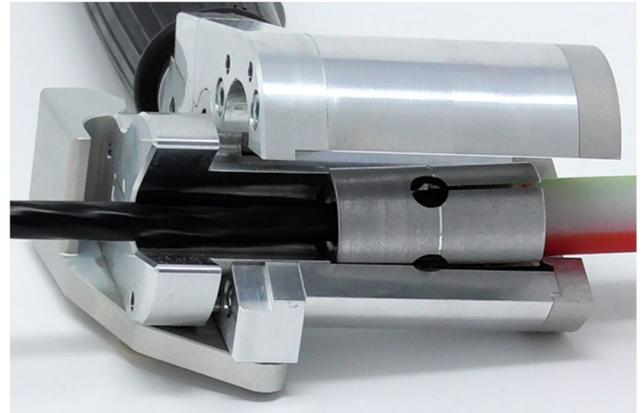
4.3 Put WGT into assembly pliers and close it. Cable has to point out top side of tool micro duct to bottom side. If it doesn't close perfect, WGT was inserted faulty.
