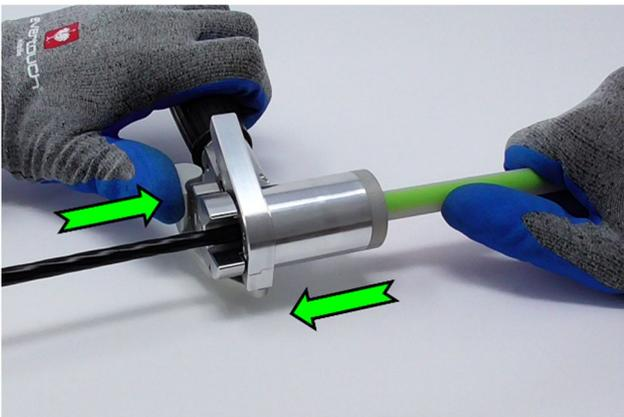
5.2 Press release lever and remove the WGT from the micro tube. Open the assembly tool and remove the WGT. If sealing gasket is clean and in good condition it may be used again.
