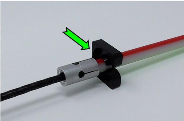
5.4 Slide PullClip on the micro duct behind WGT. The cone-shaped notch must point towards WGT.
