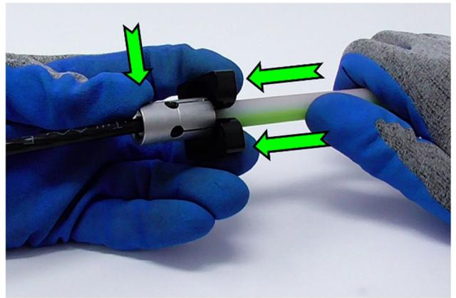
5.5 Place one finger left and another finger on right side under the PullClip, fix top side of WGT with your thumb and pull off WGT from micro tube.
