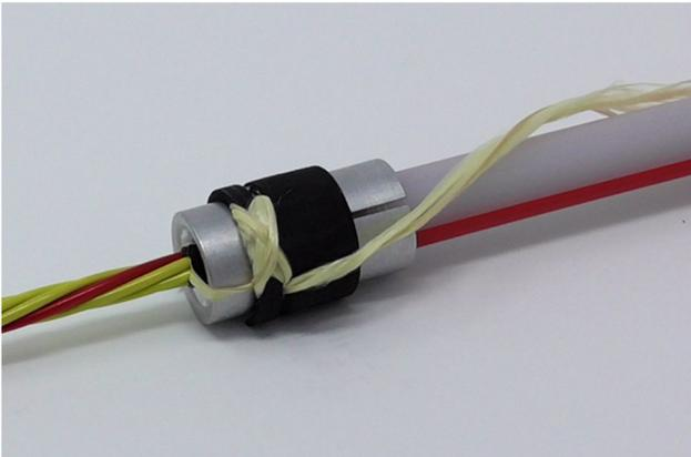
7.8 Repeat this figure 8 shape wrap up to 6 times. If possible, remain enough length of aramid yarn to enable a retry of installation.
