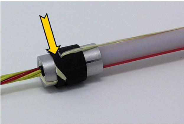
7.6 Pull aramid yarn diagonally, up to the side of the cable. Then slide it beneath flap of PowerClip back into direction of the micro tube.
