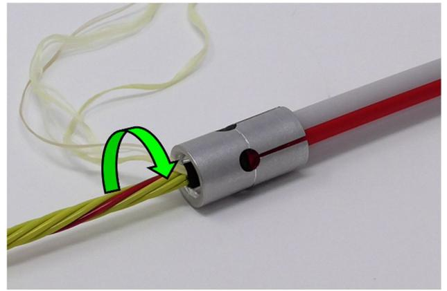
**Note:** To improve tightness and tensile strength on micro duct, rotate WGT ¼ turn clockwise. Pull aramid yarn tight and slightly twist or twirl it.
