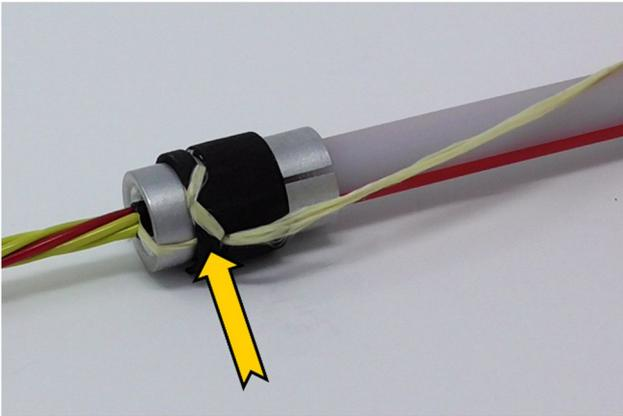
7.7 Again pull aramid yarn diagonally, upwards beneath PowerClip like described before.
