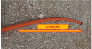
For sealing performance of permanent sealing cap it is crucial to keep at least 2m (i.e. till 1st branch) of the jacket on bundle behind cap
