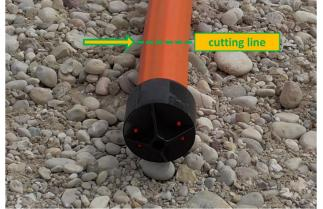
To remove permanent sealing cap, cut micro duct bundle at least 10-15cm behind the cap (cutting line). Afterwards duct bundle could be installed further as usual.
