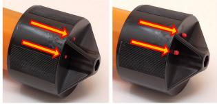
The sealing cap has control pins. In case of a 1.7 correct installation, control pins stick out of cap. Sealing compound might appear also outside of cap. This is a normal effect and has no influence on sealing performance.
