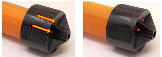
The sealing cap has control pins (patented \*) which indicate a correct installation. In case of accidentally blown micro duct, the pressure can escape at the sealing cap. Due to the self-healing effect of the sealant, the micro duct seals off itself. The permanent sealing caps have been developed for permanent underground use.
