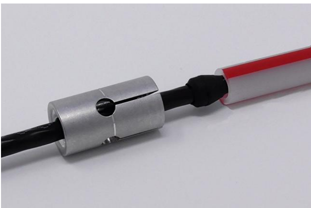
3.2 Slide sealing gasket with cone side towards micro duct onto the cable till it stops in the micro duct. Slide WGT body on cable afterwards.
